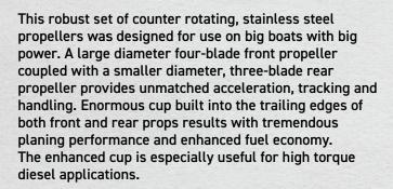
An upgrade from the standard Bravo Three propellers to the Pro Finished Bravo 3° XR props will result in one inch pitch decrease to match the same RPM. The decrease in pitch may result in 3-5 mph increase at cruise with 1-2 mph increase in top-end speed.
