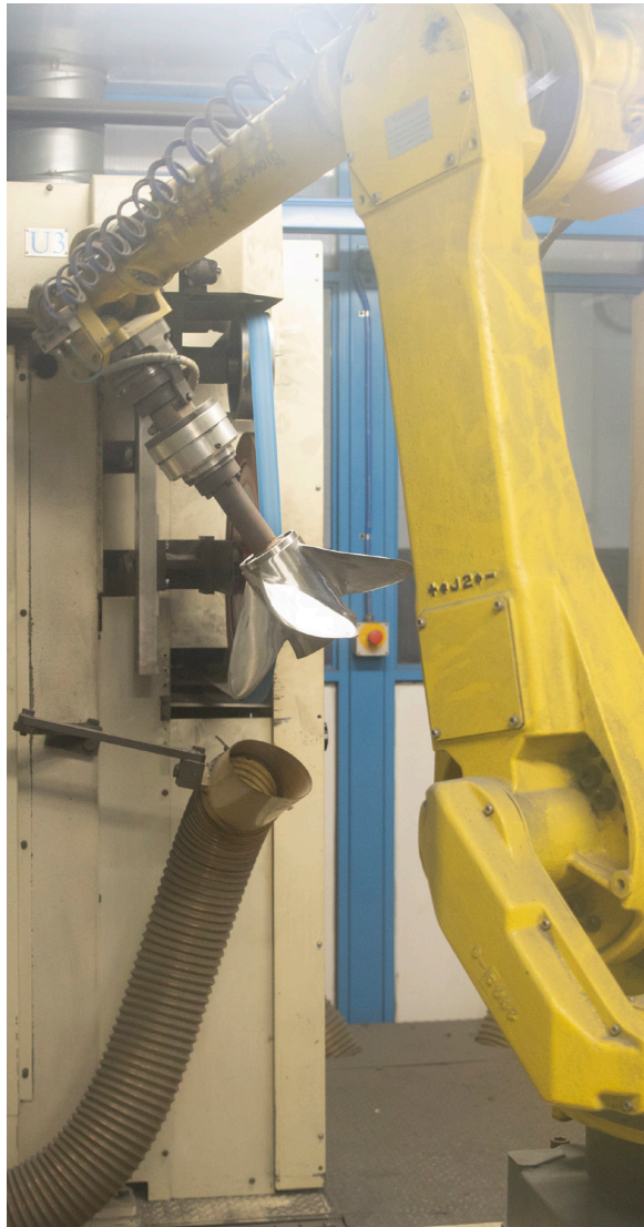
Photo above: Mercury accomplishes some grinding, machining, sanding and buffing of components using modern and energy-efficient robotic technologies. Here, a propeller is ground to meet precise specifications.
